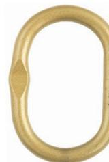
**Crosby Masterlinks A344** Made from alloy steel, quenched and tempered, then proof-tested at 2.5 times Working Load Limit [4:1]. Each link has an identification code for traceability. Masterlinks are used to create linked assemblies, such as multi-legged slings. Supplied with certification. Use 4:1 factor for chain.
