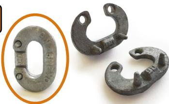
**Crosby "Missing Link" Replacement Links 6-335** Made from forged steel, quenched and tempered. Integral rivets join the two halves. After the connection is made the rivets must be peened. These joining links are not suitable for Grade 80 or 100 chain or for overhead lifting purposes. Meets or exceeds the performance requirements of US Fed. Spec. RRC-271D, Type 11, except for those provisions required of the contractor. Often used to extend or join anchor chains.
