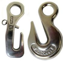
**Stainless Steel Eye Chain Hooks** Allows a temporary hauling line to be attached anywhere along a length of short link nominal 8 mm chain [which will only accept shackles on the final links]. Widely used on anchor chains to prevent snubbing by attaching a length of stretchy nylon rope which takes the strain while a loop of slack chain hangs below. Now available with a plunger. See also shortening clutches [see previous page].
