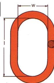
**Masterlinks Grade 80 Size 8** Available to take your own couplers or shackles. Conforms to DIN 5688-8. Supplied with certification. SPECIFICATION: Dimension 'd': 16 mm. Dimension 'w': 60 mm. Dimension 't': 110 mm. Colour: red-coated.
