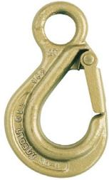
**Crosby Eye Chain Hooks with Latch M-315A** Made from forged alloy steel, quenched and tempered, then proof tested at 2.5 times Working Load Limit. Also meets proposed ASTM and Euronorm standards for Grade 80 chain fittings. Features large throat opening and integrated heavy-duty latch.
