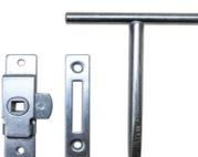
**Budget Lock** These serviceable locks are ideal for holding scenic panels in place when access behind may occasionally be necessary. If the key is lost a flat screwdriver will get you out of trouble. Often the locking arm just engages behind the stile but there is an option of purchasing a keep and also a forged T key.
