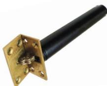
**Perko Invisible Door Closer** The cylinder is mortised into the inner edge of the door, a chain links the cylinder spring to an anchor plate fitted to the door frame. Easy to install, suitable for light to medium weight doors.
