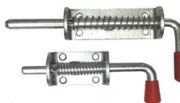
**Spring Bolts** A strong spring loaded bolt which can be held in the retracted position by twisting the bolt through 90°. Available in two sizes. Fixings: 4 off M6 csk machine screws.
