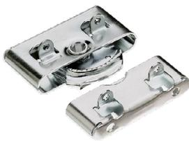
**Concealed Shallow Tab Butt-Joint Latch** Similar to the Roto Lock fastener above, however the latch and receptacle are secured with the tabs on the housing instead of the entire assembly mounted into the panel. Especially useful for quickly fitting flats and rostra. The latch and receptacle each require a 88 x 17 mm mortise in the panel 88 x 17 x 19 mm deep. These are exact sizes so some clearance may be needed. This tab mounted assemblies should be mounted with M5 screws [see page 265].
