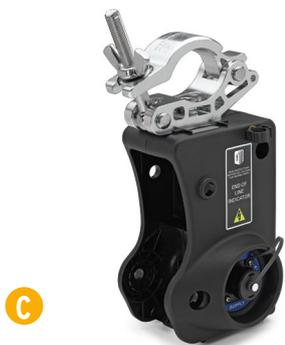
**End of Line Unit** This unit forms part of the circuitry which proves electrical continuity in the cabling. Only used in conjunction with the Sensing/DMX Firing Unit. The unit has three switches, all of which should be on for a single chain of Kabukis. Individual switches should be used when two or three chains of Kabukis are used in conjunction with the splitter box. A green LED on the unit indicates the cables are correctly connected.
