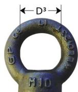
**Eye Nuts** Made from C15 carbon steel to Din 582 with a safety factor of 4:1. Other sizes available to order. Self-colour.
