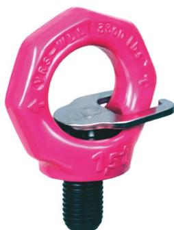
**Starpoint VRS F** Often referred to as "Pink Ladies". The pull on most eye bolts has to be restricted to the plane of the eye but the Starpoint VRS adjusts through 360° to align with the direction of pull. The star-shaped design and striking fluorescent pink powder coating clearly distinguishes it from other eye bolts. Each bolt has a clear WLL
