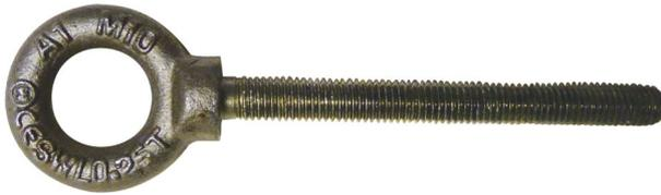
**Long Shank Dynamo Eye Bolts** Commercial quality drop forged eye bolts, intended to fix through a surface material with a hex nut to provide a single fixing point. The load must be a vertical pull and the bolt must be tightened down to the shoulder. Self-colour.
