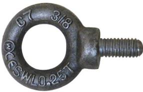
**Short Shank Dynamo Eye Bolts** These eye bolts are primarily designed to go into tapped holes. The manufacturer's SWL will only apply if the tap depth is the full threaded length plus
