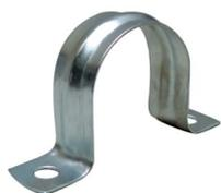
**Galvanised Pipe Clips** These always cause mass confusion because they are labelled according to the nominal bore of the pipe! So a 1 1/2" clip fits a 2" outside diameter pipe. The trouble was some of you knew that! Our little table below should
