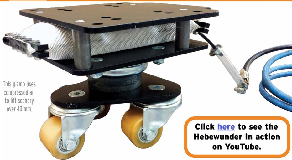
This gizmo uses compressed air to lift scenery over 40 mm.
