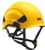
**Petzl Vertex** Replaces the Best and the ST A12. A traditional style industrial helmet with no ventilation holes for extra protection. Ideally suited to prolonged or regular work with electricity where the hard shell will safeguard against sparking. Conformity: CE, EN397, EN12492, EN50365, ANSI Z89.1 Type 1 Class E, EAC, AS/NZS1801: meets all requirements of EN 12492 standard, except the ventilation requirement. May be eligible for zero rate VAT [page 339].
