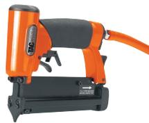
**Tacwise A7116V Pneumatic Stapler** A professional fast reliable gun suited to the full-time coverer/canvasser. SPECIFICATION: Takes up to 180 Type 71 staples from 4 mm to 16 mm. With a quick release fitting which fits our 9 mm bore hoses. Air consumption: 1.6 cfm. PSI: 60 - 100. Max 77 dBA on impact. Supplied in a handy plastic carry case.
