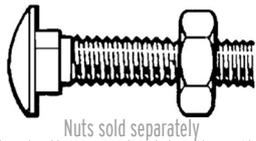
**Coach Bolts [Carriage Bolts] DIN 603/555** Intended as a fixing for a wooden surface, either wood-to-wood or wood-to-metal.
