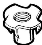
**T-Nuts** Simply drill a hole in your timber to accommodate the shank of this fitting and hammer it home! It provides a captive nut that is held in place by the prongs. Ensure that you fix the nut so the bolt pulls against the prongs.
