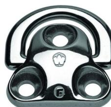
**Folding Pad Eye** Drop-forged with no welding to offer remarkable strength. In addition, by aligning the D-ring to the direction of the force they can handle higher operating loads. Often used to secure trapeze tension wires. A small silicone pad included can be used to when folded flat. Also available in titanium.
