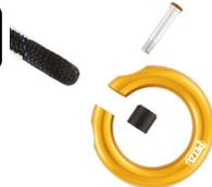
**Petzl Ring Open** An aluminium manual locking attachment with massive scope as a semi-permanent connection for PPE, or for joining wires or ropes. The plastic spacer unfastens using the supplied 3 mm Allen key and leaves an 11 mm opening wide enough to take rope with sewn terminations. Tighten the pin following maker's instructions for 23 kN on all axes. Conformity: CE EN 362: 2004/M
