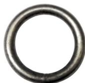
**Steel Welded Rings [self-colour]** Useful for a multitude of purposes including lightweight multi-legged suspension, heavy-duty curtain rings and useful securing points when used with Grummets [page 148]. They are supplied self-colour so they can be welded directly to steel work or cut open and re-welded. For lifting purposes use Rated Shackles [page 180] or Masterlinks [page 195].
