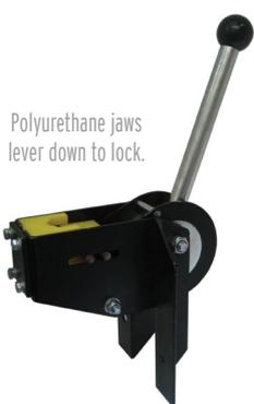
**Lever Rope Lock with Polyurethane Jaws** Handles 20 mm diameter three- or four-strand ropes. The polyurethane jaws have been designed to reduce damage to the hauling lines. On this version the lever is pushed down to lock the rope. It also has a clip to secure the handle in the free running position. Proof-tested to 100 kg using four-strand hemp.
