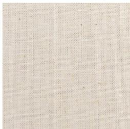
**Calico 195 g/m<sup>2</sup>** NDFR. Natural colour. A good economical lightweight material suitable for covering plywood clad flats. Calico, being rather lightweight, will not disguise poor joints between ply sheets which may need filling [see pages 49-50 for suitable fillers]. If the surface is very poor, cotton
