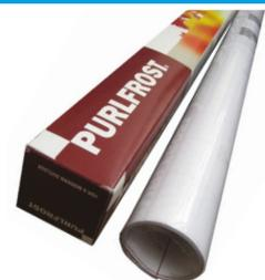
**Frost Film [Purlfrost]** Self-adhesive clear frosted films for obscuring windows. To apply, wet the adhesive side with soapy water, apply to the window, and squeegee [see page 141 or 362 for squeegees] out any bubbles from the centre outwards.
