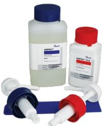
**Ampro Handipack** This convenient little pack is perfect for small props and general repairs. It consists of resin, hardener and dispensing pumps. simply pump 3 pumps of resin to 1 pump of hardener for the perfect ratio to mix. Complete with instructions, this high clarity, and low-temperature curing pack will prove invaluable in any props workshop.
