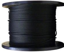
**Black Wire Rope [BS EN 12385-4] [Steel Core] 1,770 N/mm<sup>2</sup>** These popular matt black flexible wire ropes are suitable for use as running rigging whereas the PVC-coated cables listed above should not be used over pulley sheaves. Not suitable for use outdoors.
